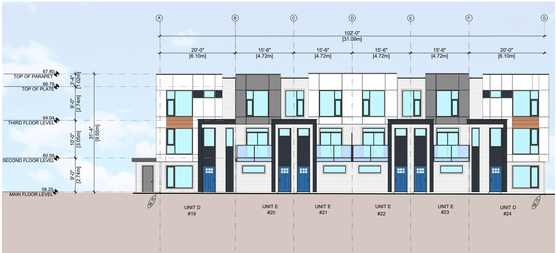
2 BUILDING 4 SOUTH ELEVATION
