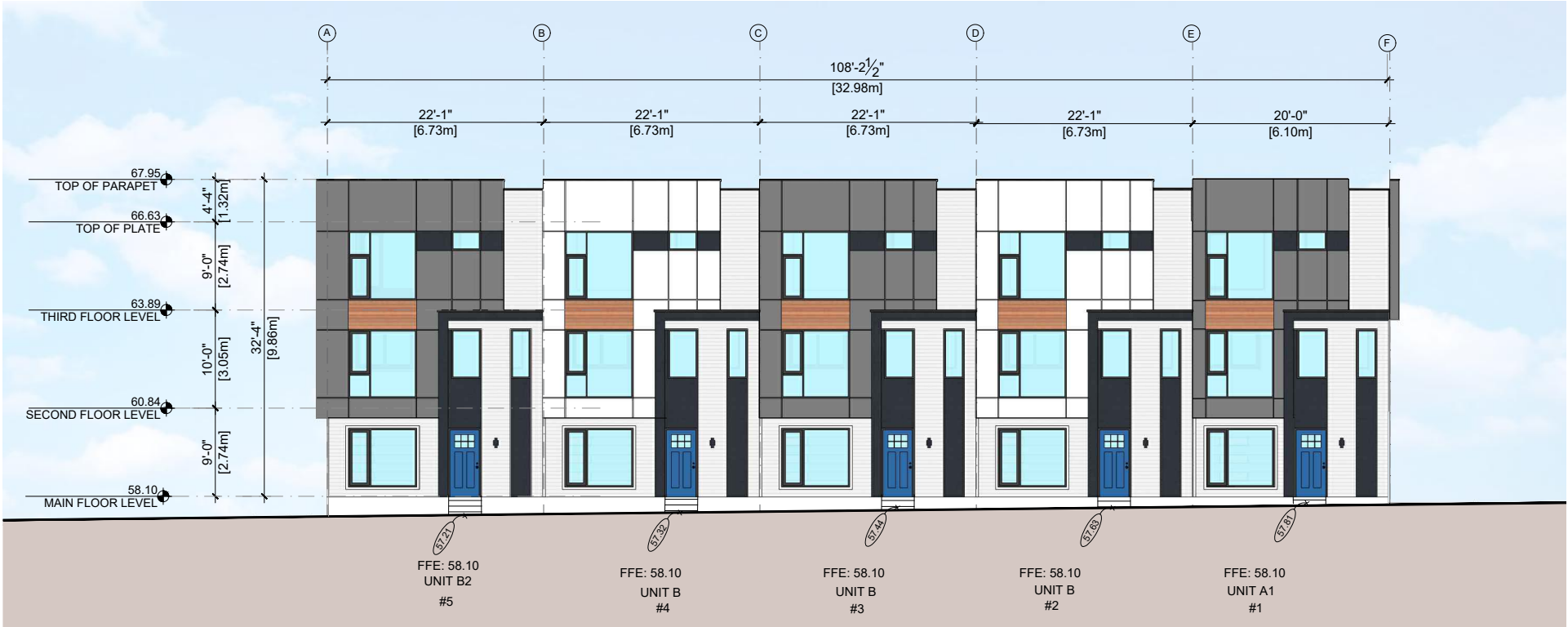
1 BUILDING 1 WEST ELEVATION
