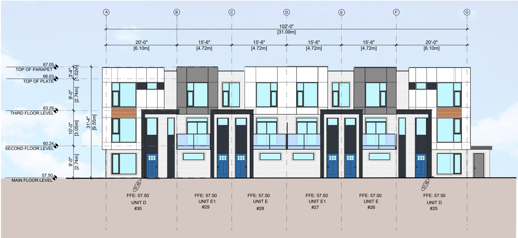
2 BUILDING 5 EAST ELEVATION
