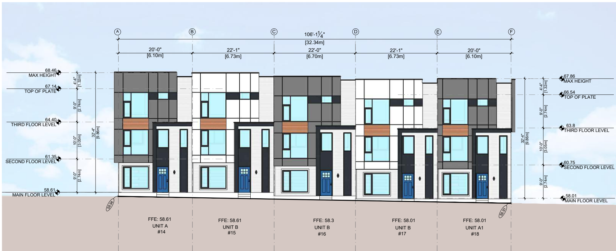
2 BUILDING 3 SOUTH ELEVATION
