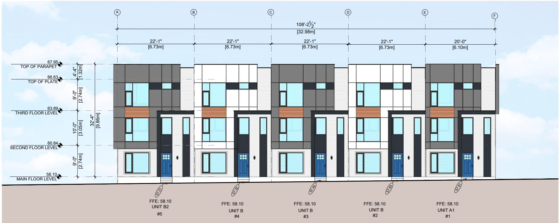
1 BUILDING 1 WEST ELEVATION
