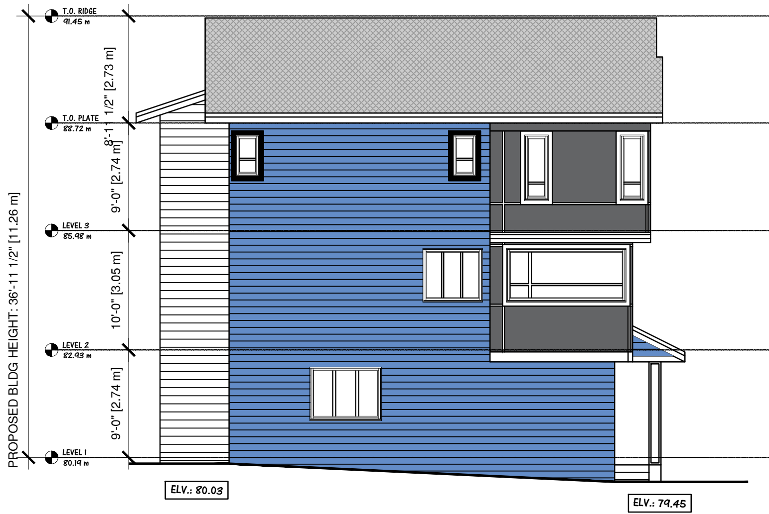
BUILDING 8 (EAST ELEVATION)
