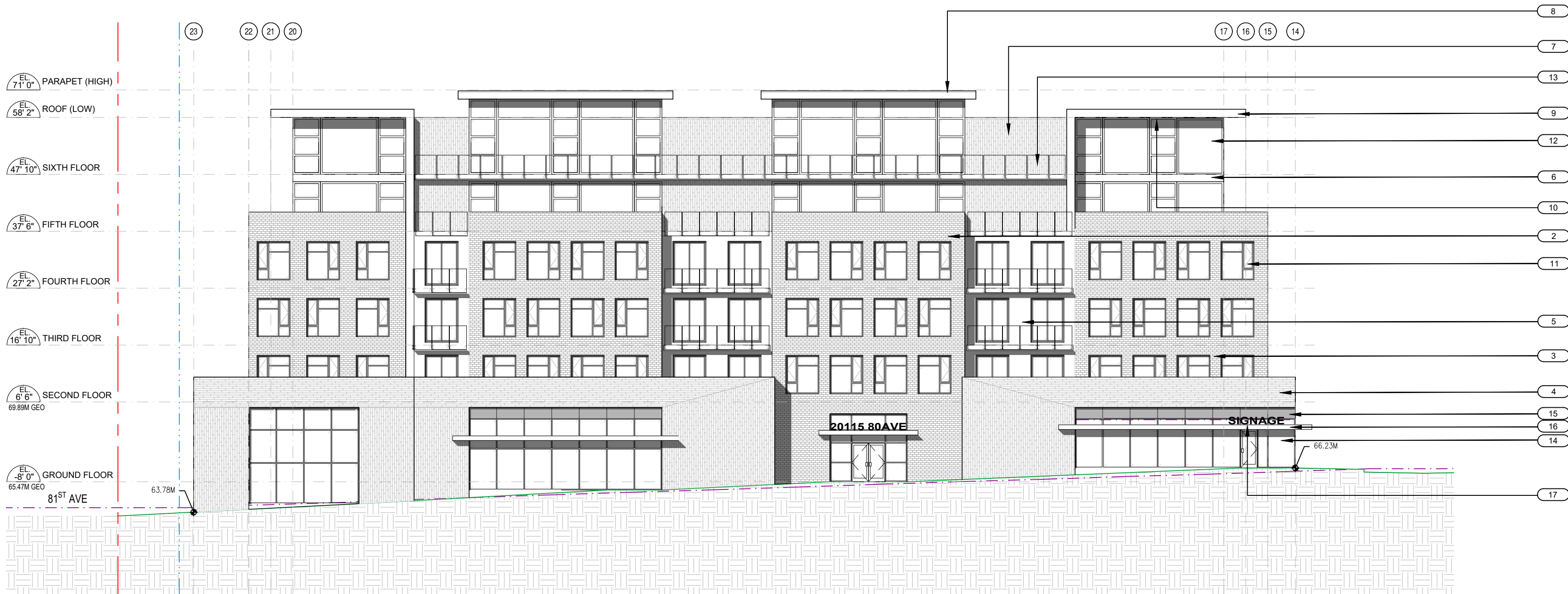
B1 ELEVATION: WEST (FRONT) 201 ST 1/16" = 1'-0"
