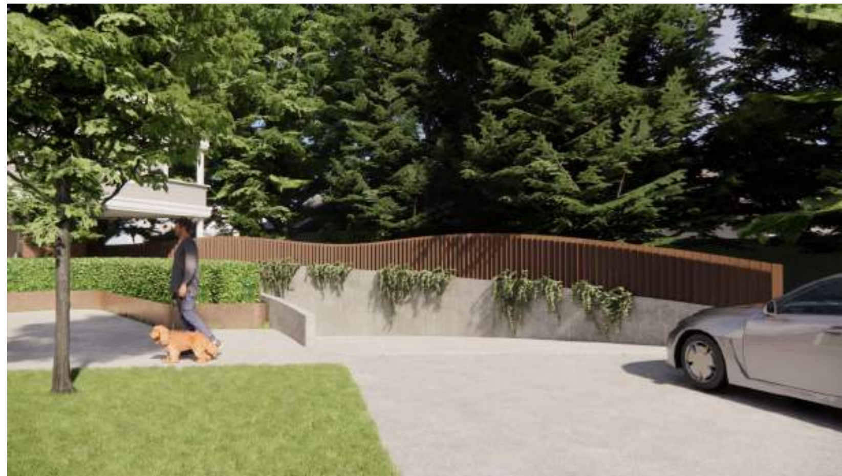
4 WOOD SLAT SCREEN BLOCKS VEHICLE LIGHTS COMING IN AND OUT OF PARKADES
