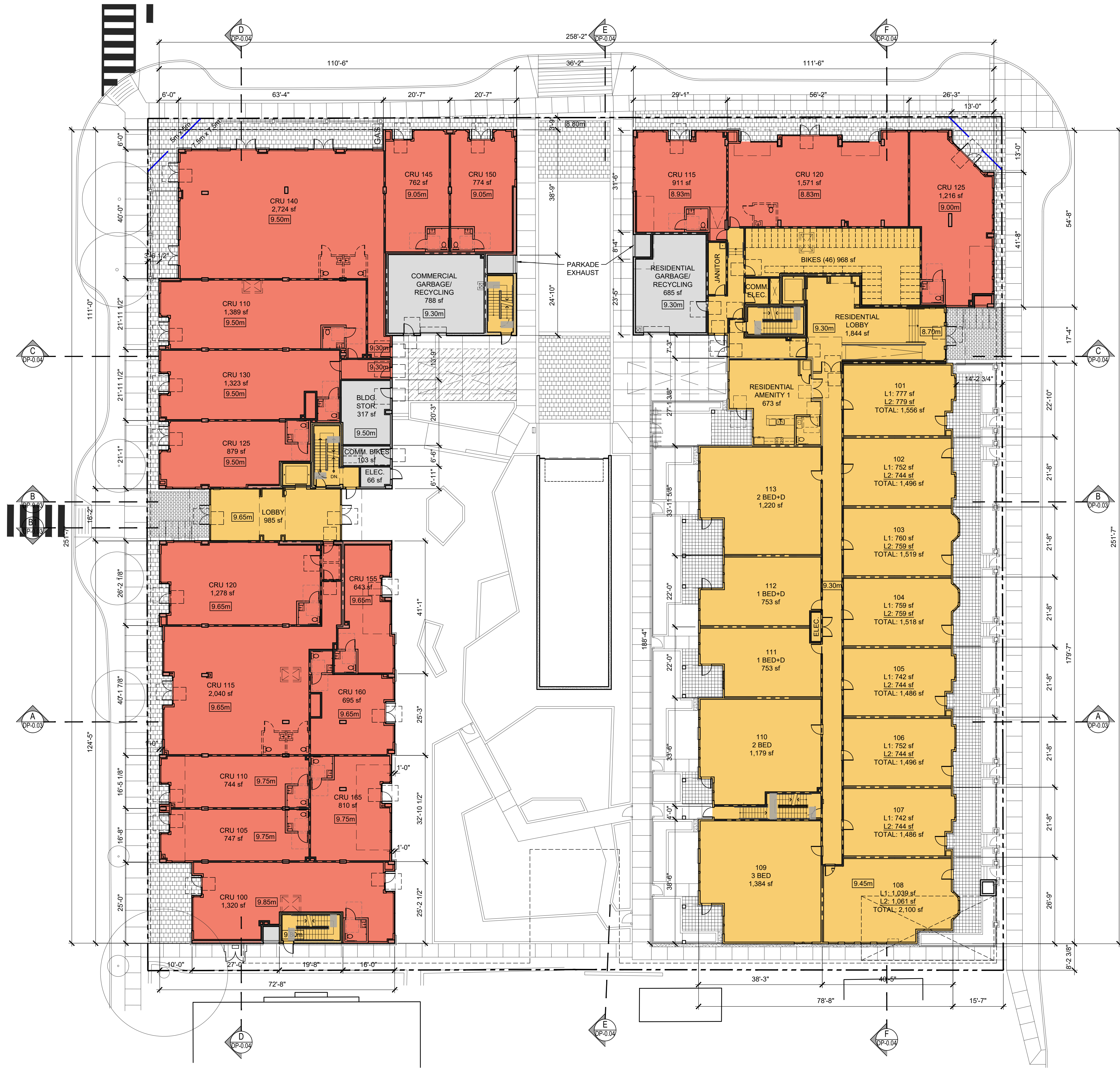
MAIN FLOOR PLAN (FLOOR AREA: 39,541 GSF) SCALE: 1/16" = 1'-0"
