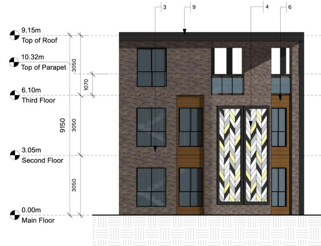
6 NORTH ELEVATION - (AMENITY BUILDING) Scale: 1:100
