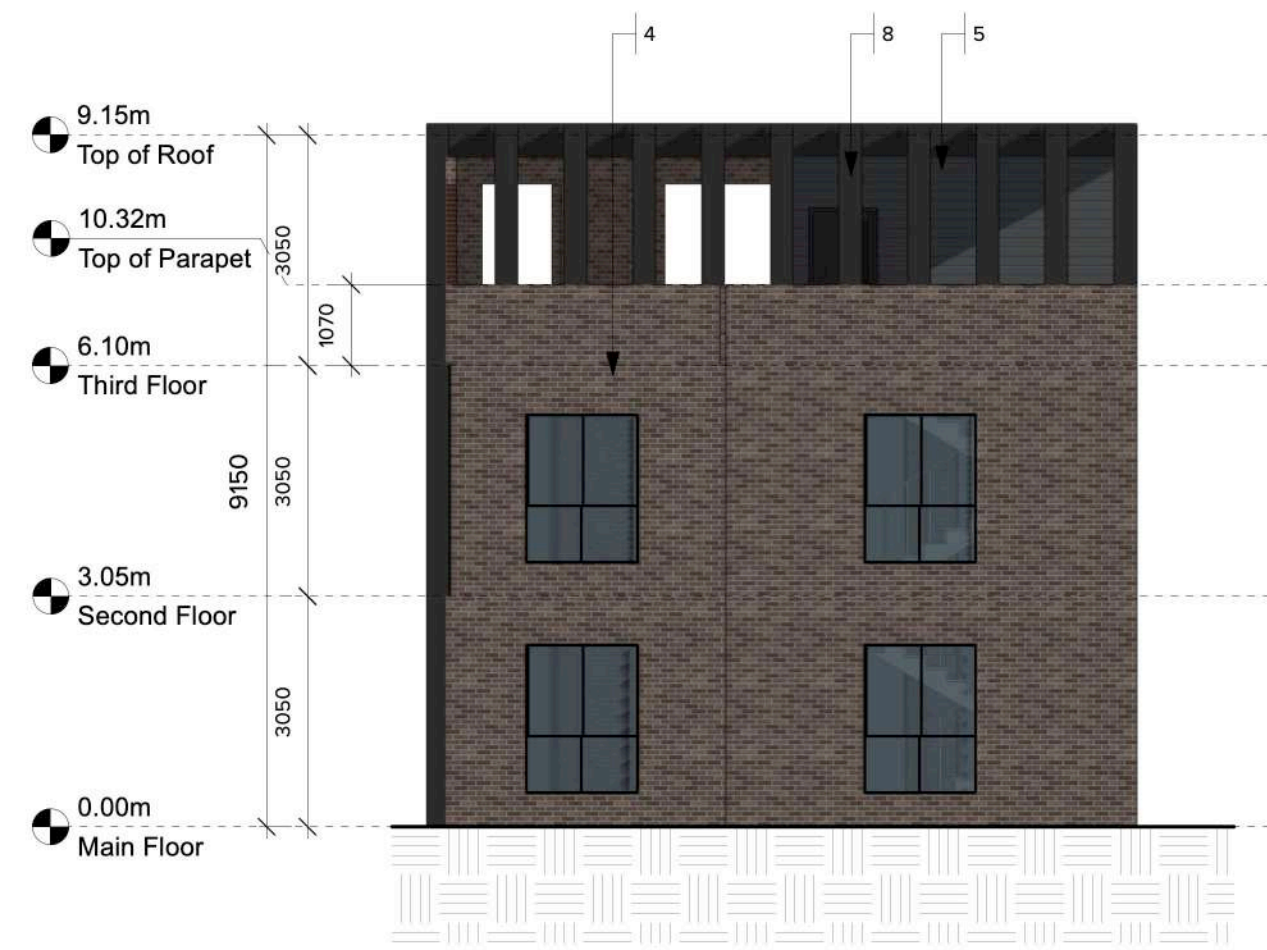
8 SOUTH ELEVATION - (AMENITY BUILDING) Scale: 1:100
