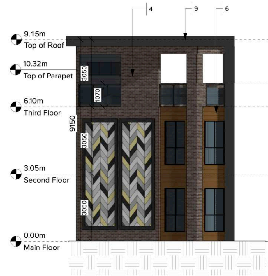
5 WEST ELEVATION - (AMENITY BUILDING) Scale: 1:100
