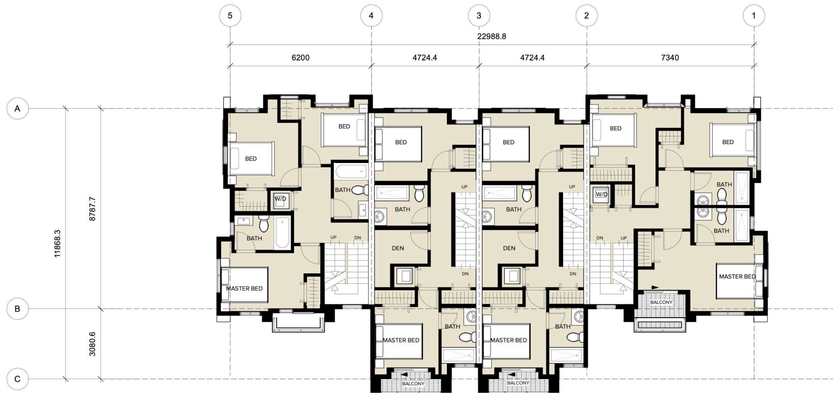
3 BUILDING 6 - THIRD FLOOR PLAN Scale: 1:100
