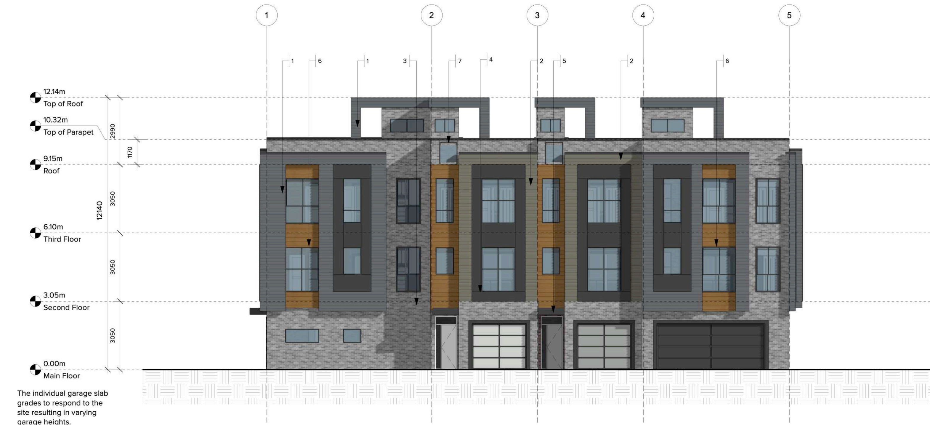
1 NORTH ELEVATION - (BUILDING 5) Scale: 1:100
