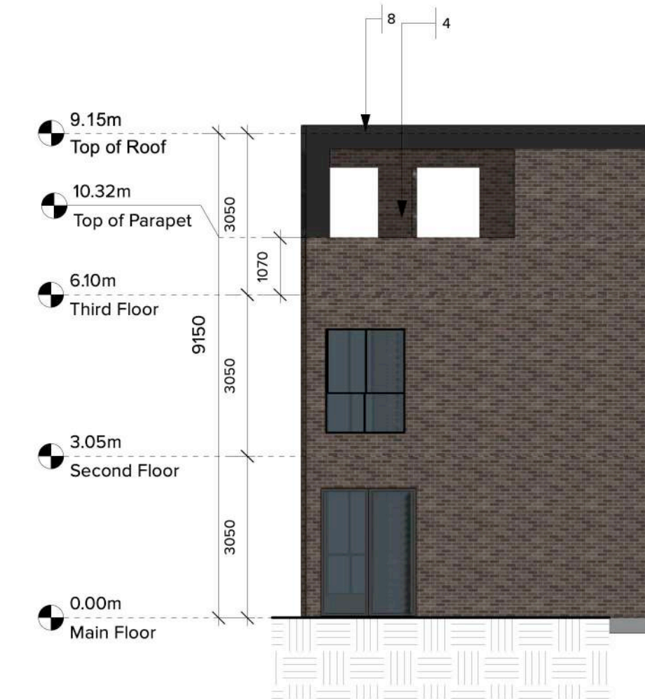
7 EAST ELEVATION - (AMENITY BUILDING) Scale: 1:100
