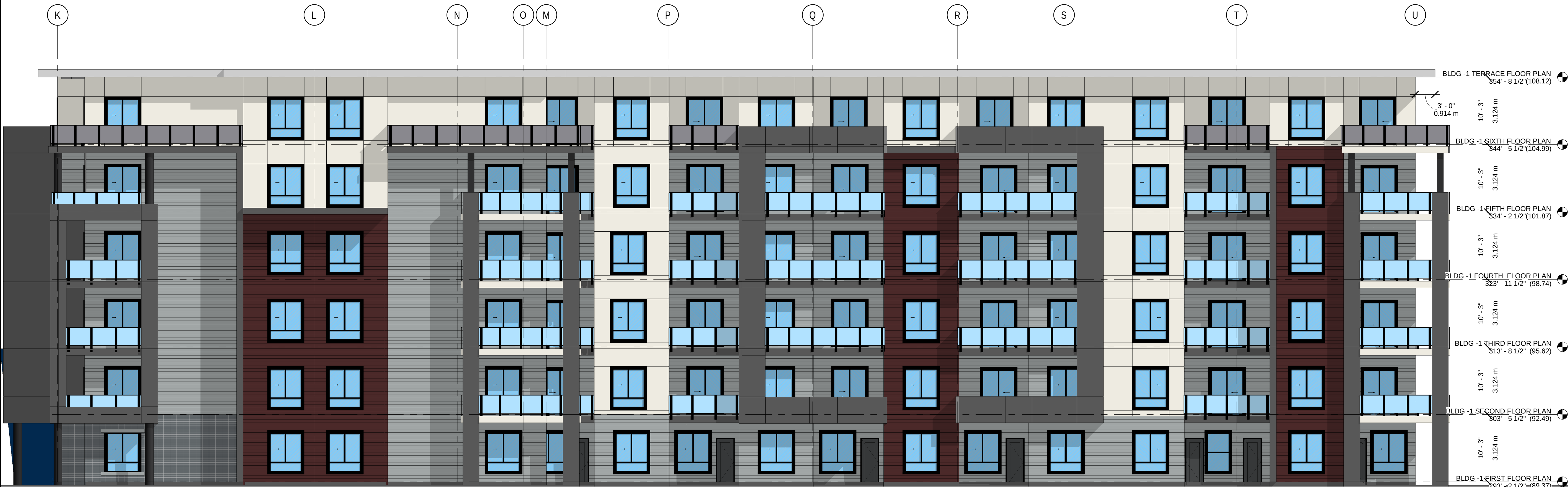
1 BUILDING 1 COURTYARD SIDE A-302 SCALE: 1/8" = 1'-0"
