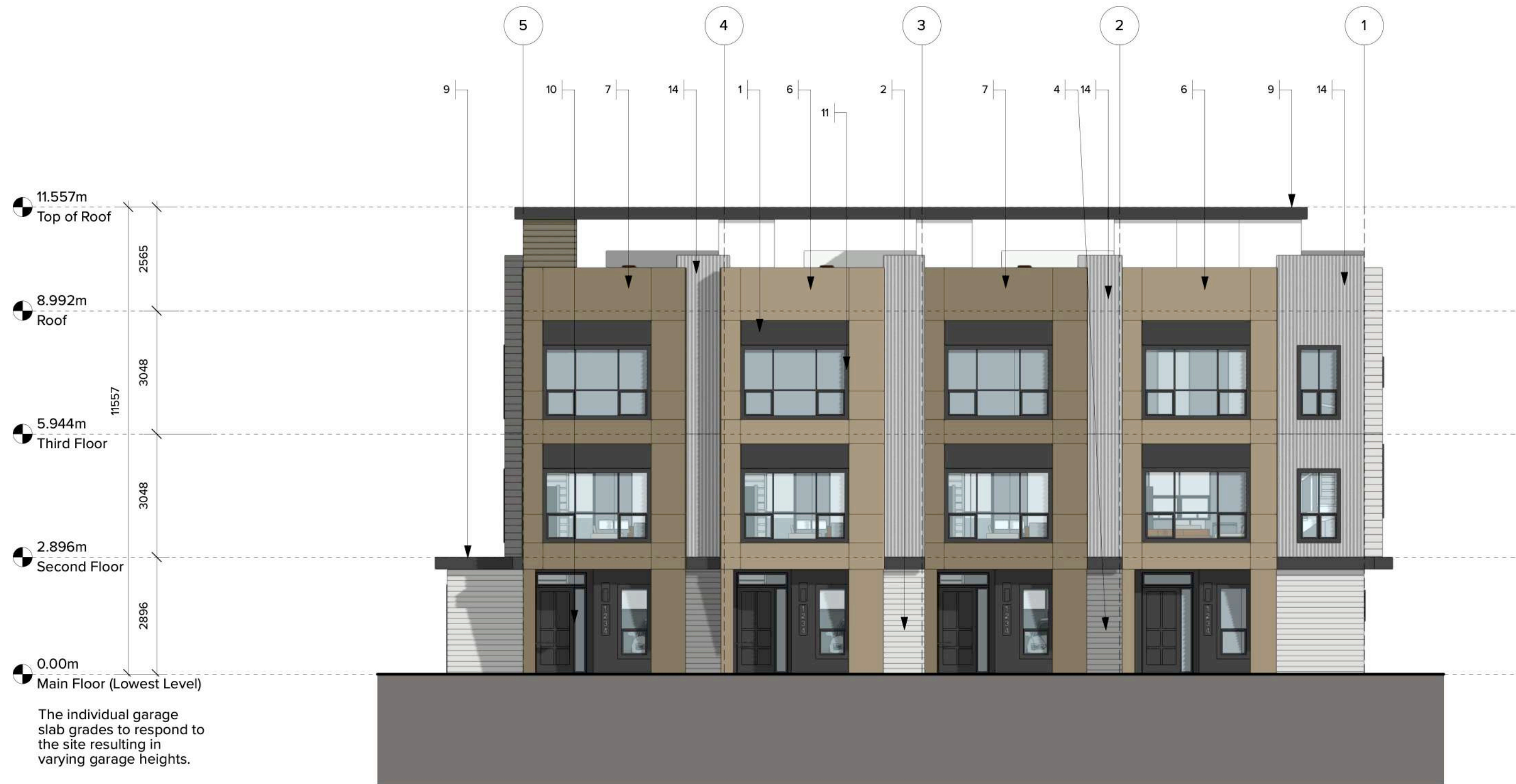
1 BUILDING 5 - SOUTH ELEVATION Scale: 1:100
