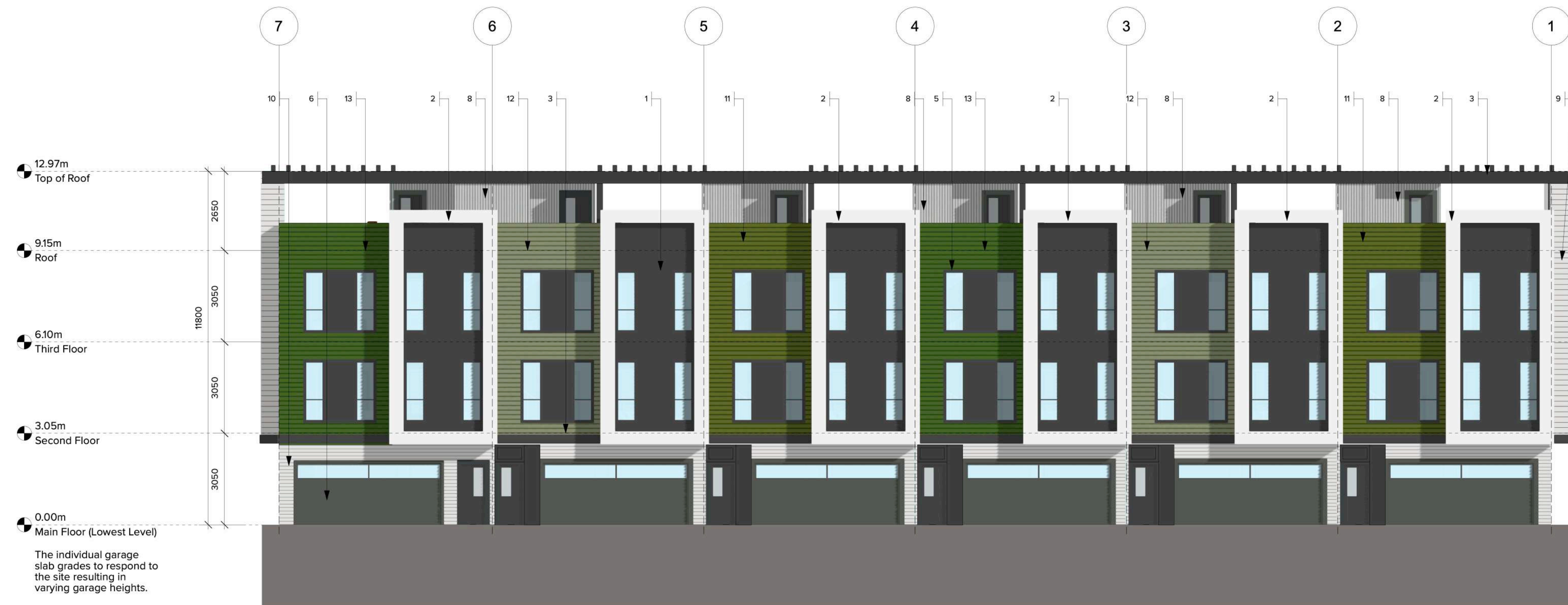
2 BUILDING 6 - NORTH ELEVATION Scale: 1:100
