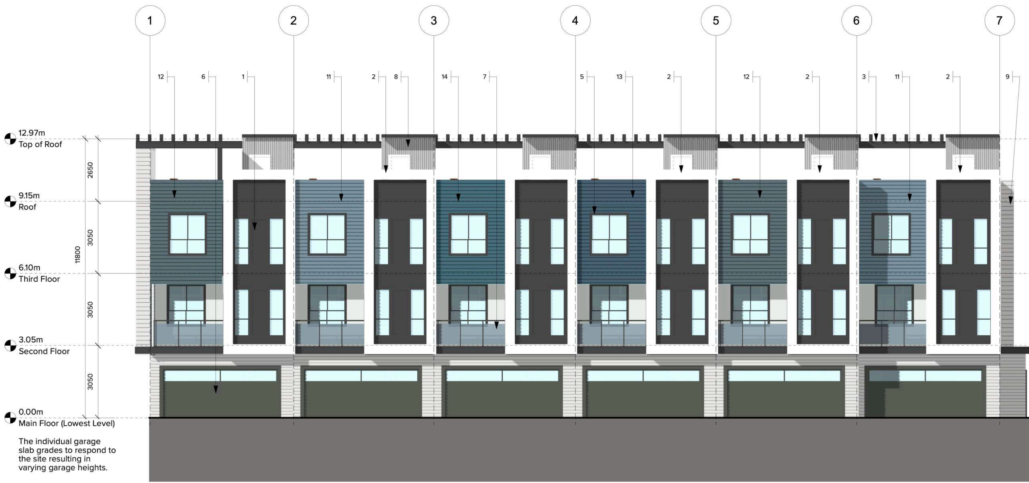
2 BUILDING 4 - WEST ELEVATION Scale: 1:100
