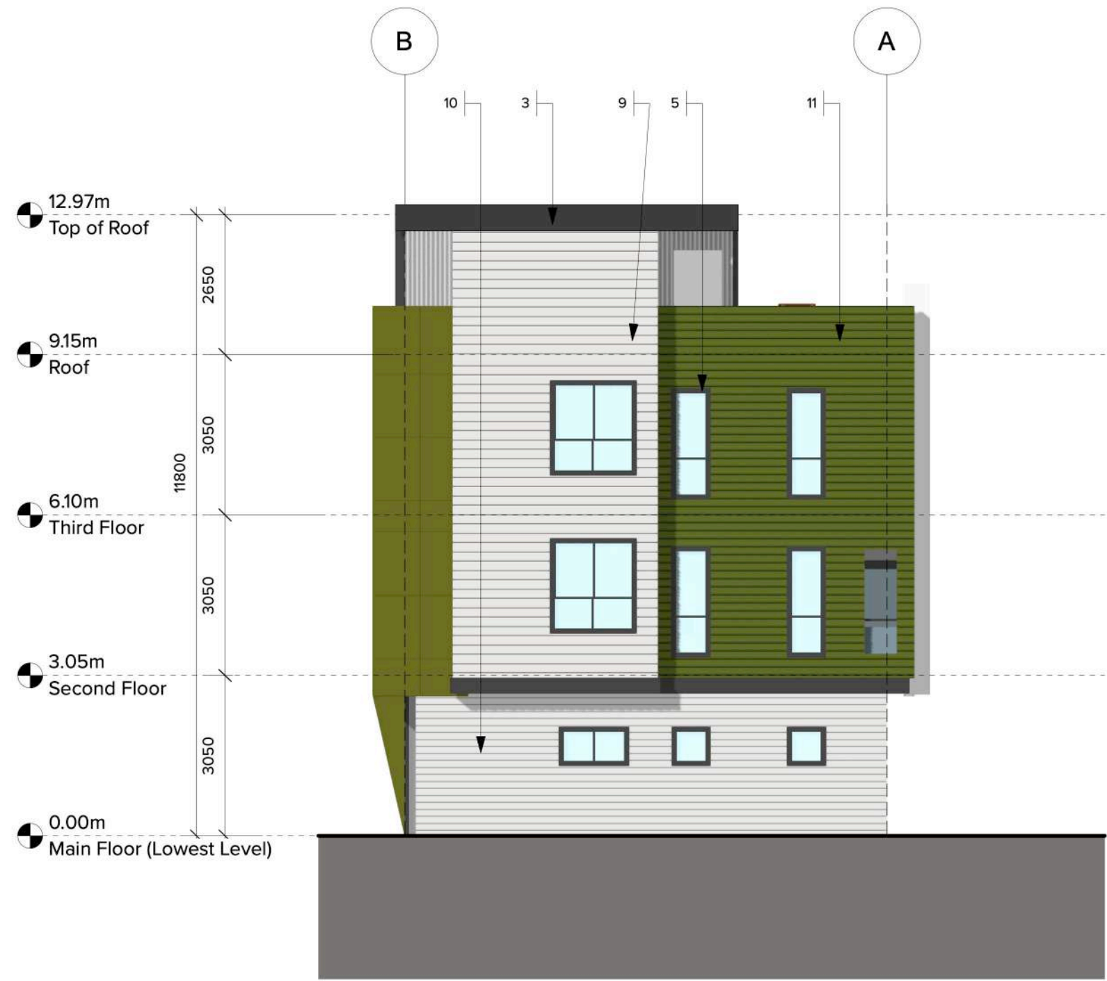
4 BUILDING 8 - SOUTH ELEVATION Scale: 1:100
