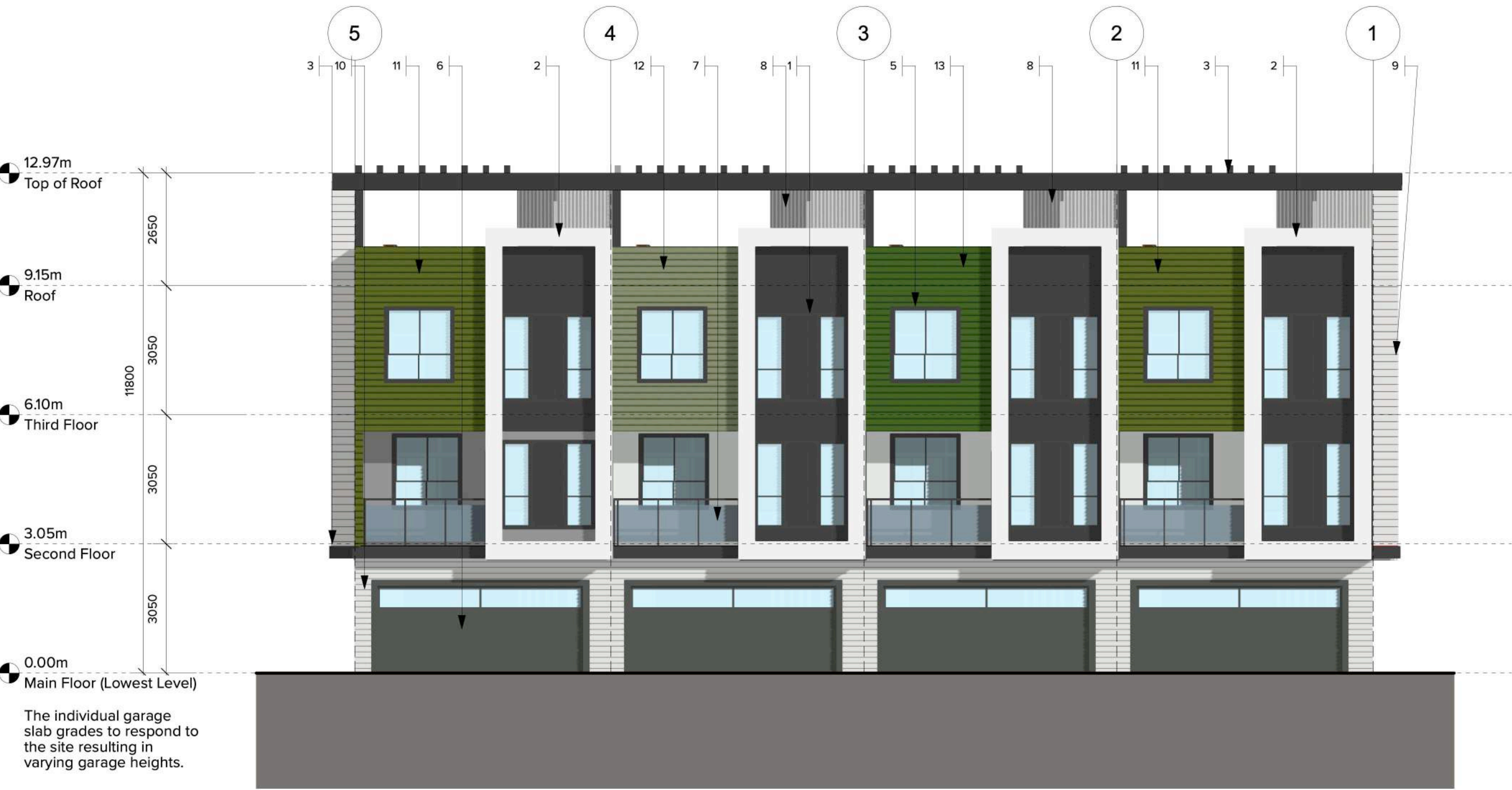
2 BUILDING 8 - EAST ELEVATION Scale: 1:100
