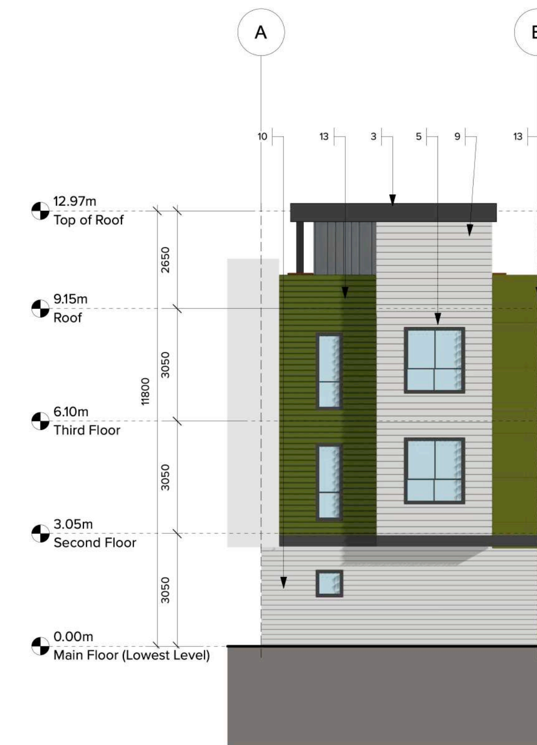
4 BUILDING 6 - WEST ELEVATION Scale: 1:100
