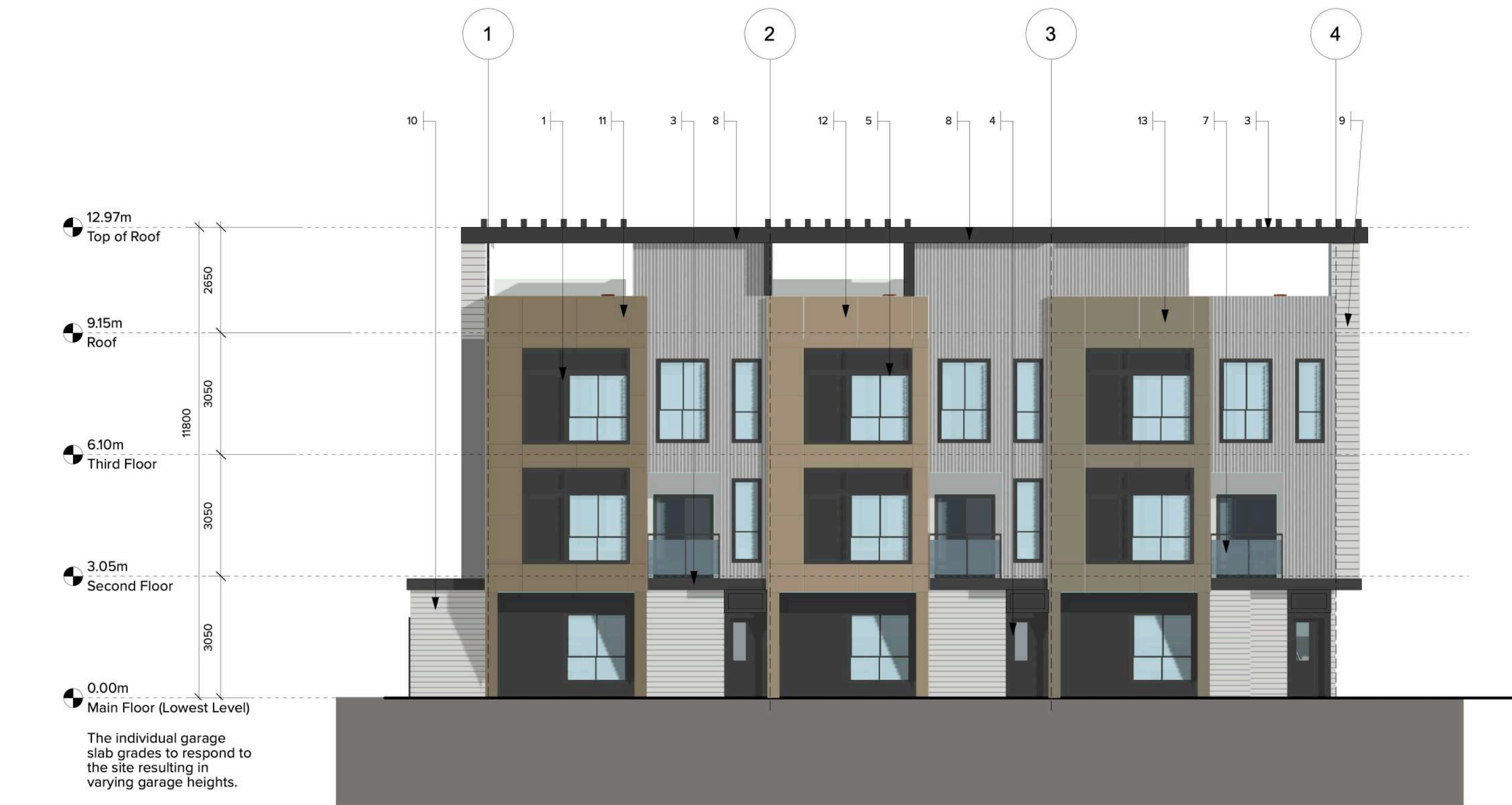
1 BUILDING 5 - SOUTH ELEVATION Scale: 1:100
