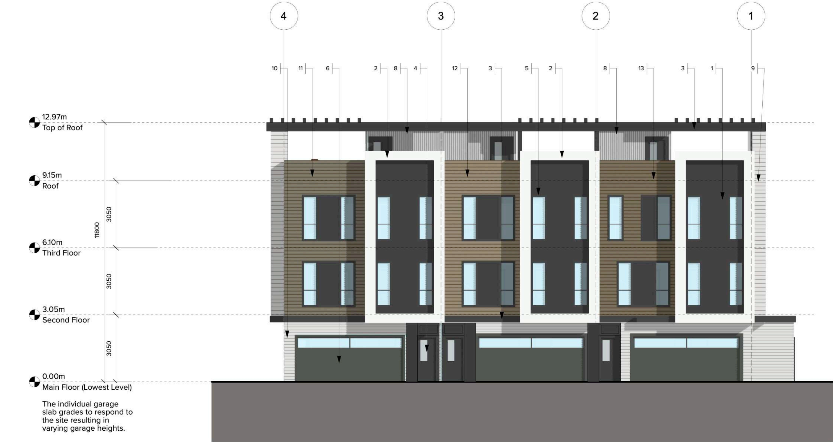
2 BUILDING 5 - NORTH ELEVATION Scale: 1:100
