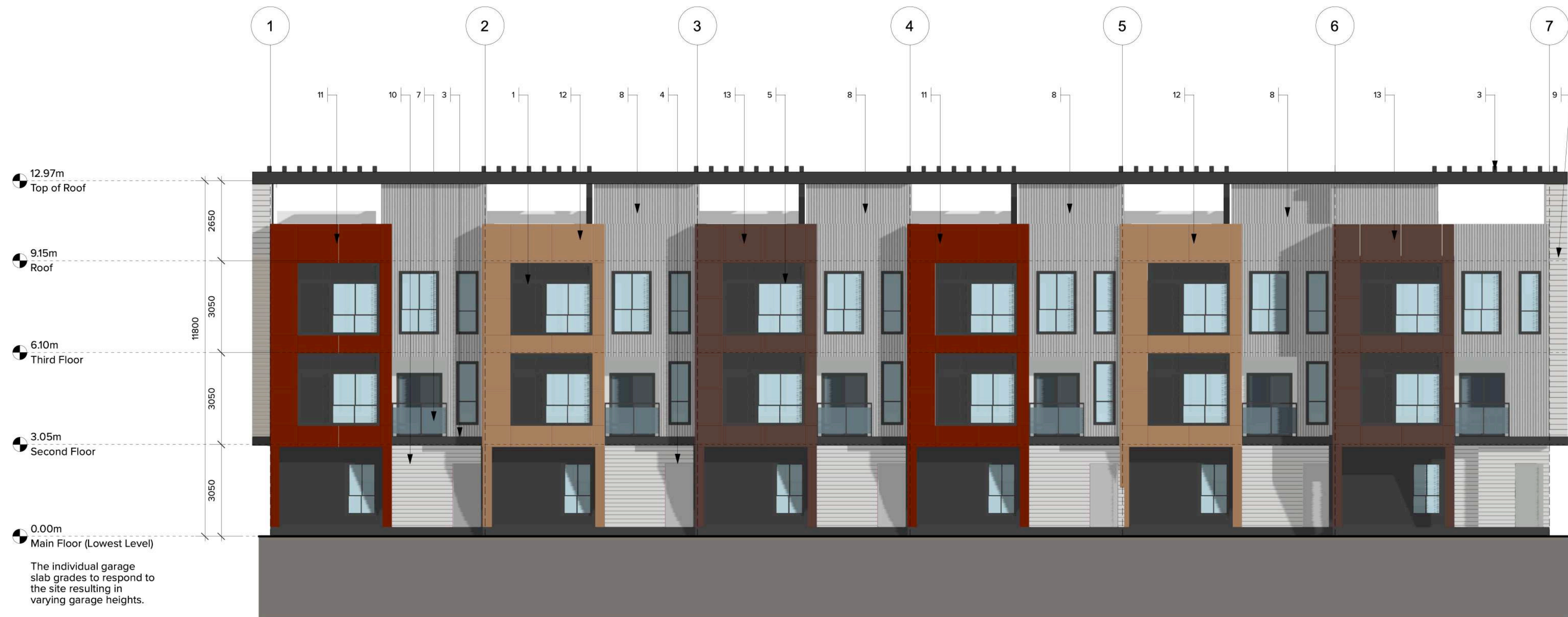
1 BUILDING 7 - SOUTH ELEVATION Scale: 1:100
