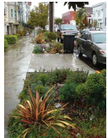
Figure 39. Storm water source controls like these rain gardens reduce pollutant run-off.
