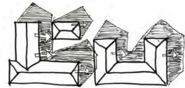
Figure 18. Corner and through units facilitate natural ventilation and daylight access.
