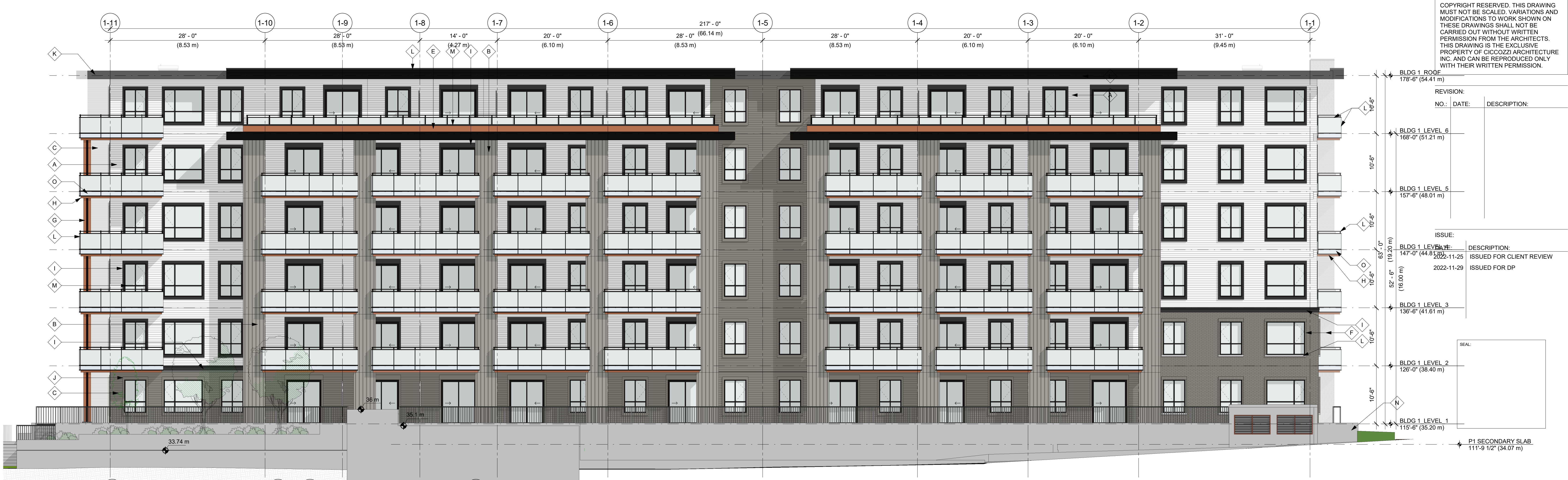
2 A4.0 BLDG 1 - ELEVATION WEST_DD 1/8" = 1'-0"
