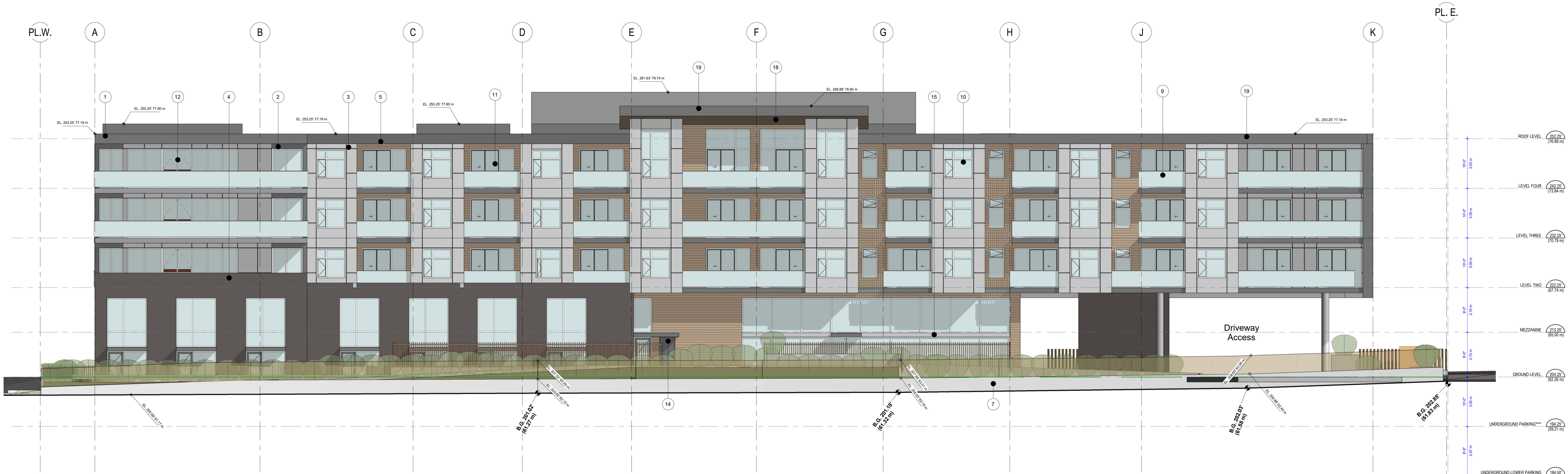
1 DP SOUTH ELEVATION 1/8" = 1'-0"
